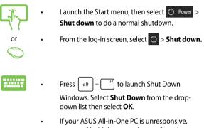
press and hold the power button for at least four (4) seconds until your ASUS All-in-One PC turns off.
