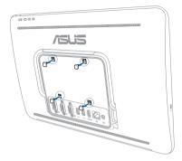
3. Attach the four wall mount screws to the rear panel holes.
